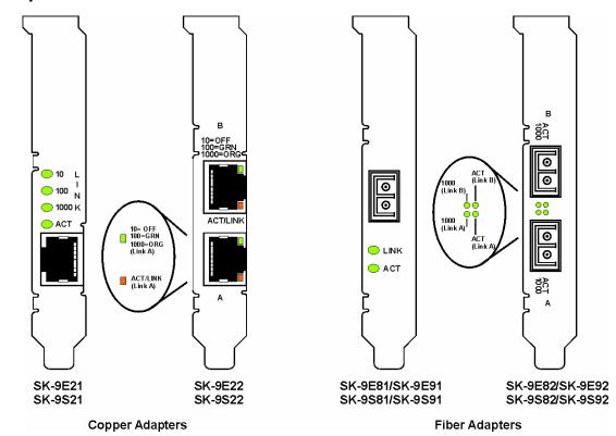
Figure 5. Location of the LEDs (adapter variant 2)
